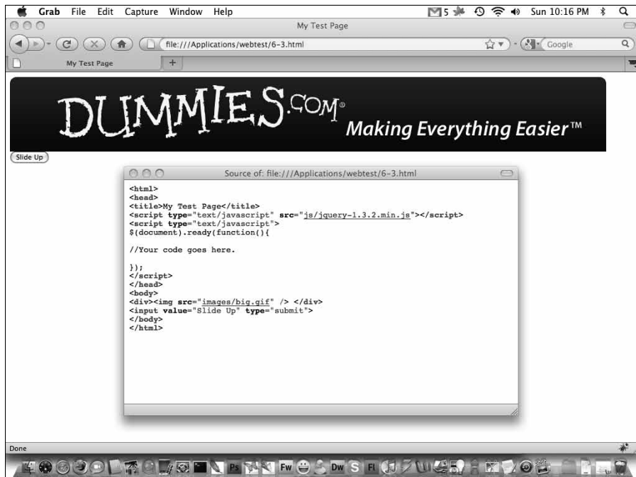
Figure 6-3: Web page with a button and a <div> element containing an image.
